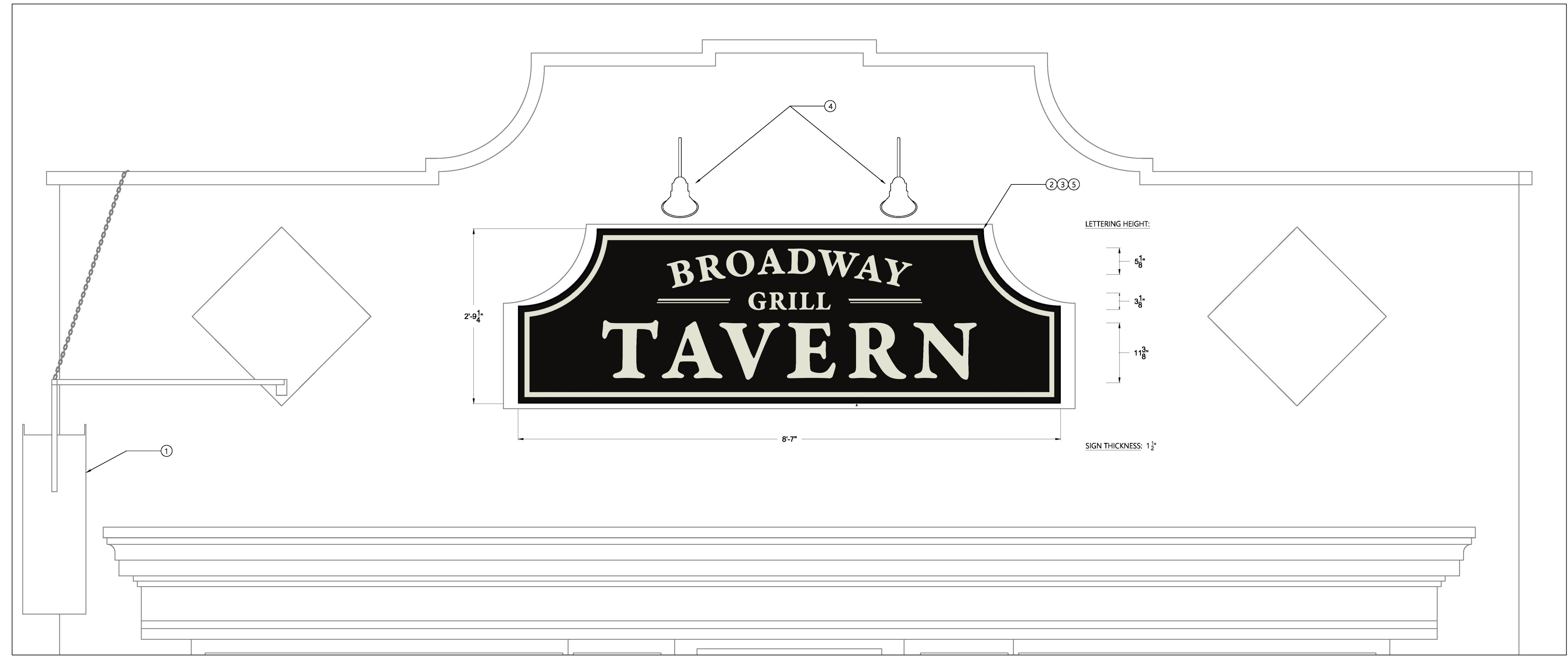
1 PROPOSED SIGNAGE W/ DIMENSIONS SCALE: 1"=1'-0"
